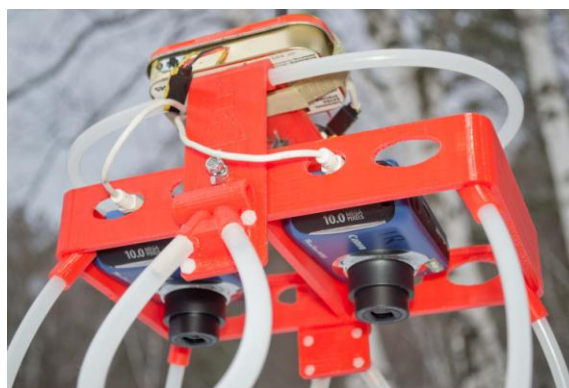
The Titan 2 Rig with normal and infrared Canon A495s and external shutter trigger electronics on the shoulders of the upper frame. USB cables reach the cameras through oval windows.
