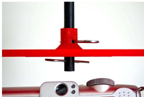
The upper cotter pin prevents spinning and the lower pin can prevent disaster.
