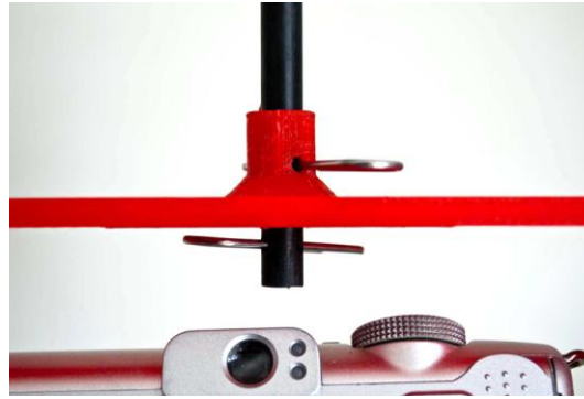
The upper cotter pin prevents spinning and the lower pin might prevent disaster.
