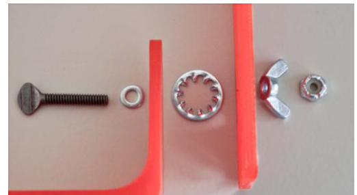
The large toothed lock washer goes between the camera tray and the upper frame. The wing nut and lock nut go on the outside of the frame.
