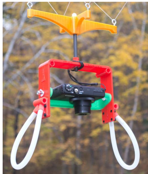
Use the small tray for flights with one camera. The camera wrist strap is used as a safety lanyard.
