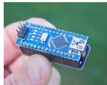
Press the reset button (white, center left) on the Nano to activate a new mode that has been selected with the DIP switch.
