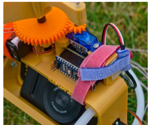
The 8" strap wraps over the servo bracket. Its free end can hug the Velcro of the camera cable which can hug the front of the 8" strap.
