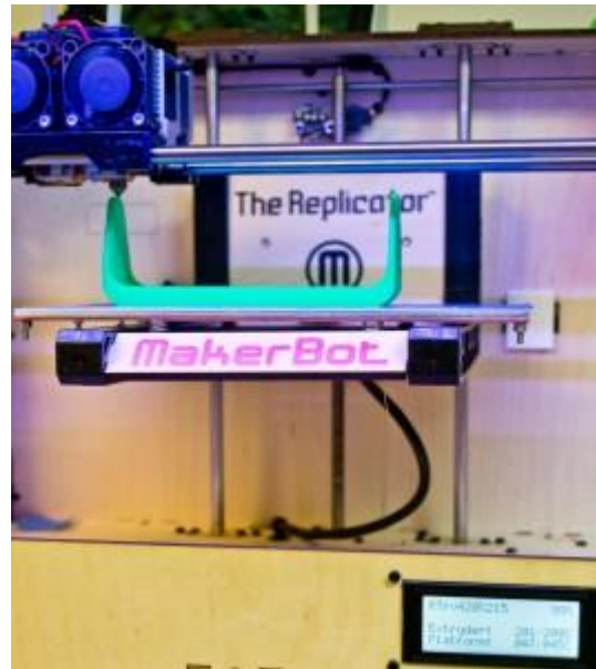
The MakerBot Replicator just finishing a standard tray for the Redstone Rig.
