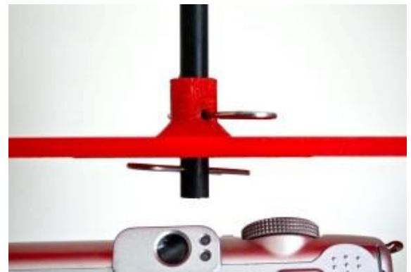
Both cotter pins are required.
