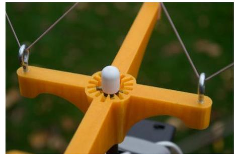
*The star allows the camera rig to be pointed in 16 directions.*
