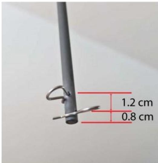
*Drill or grind two holes near the lower end of the shaft.*
