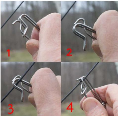
1. Attach the KAP'n Hooks about five or six feet apart on the flying line. (Adjust the clips with pliers for a better grip on thin line.)
