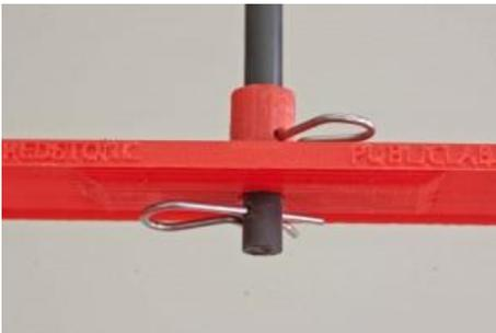
1. Insert the shaft into the bracket on top of the camera rig frame and insert a cotter pin through the lowermost hole until the pin locks.
