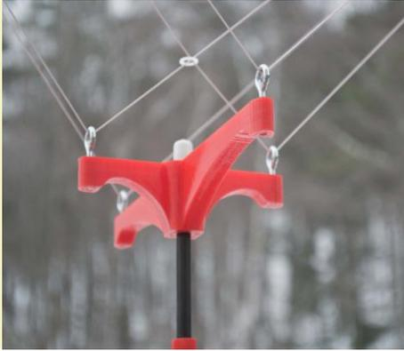
The Picavet is the most popular camera suspension system with kite aerial photographers. The Picavet system has two attachment points at the kite line about five feet apart which reduce rotation of the rig and swinging along the axis of the kite line. The Picavet lines pass freely through four eyes on the Picavet cross, and the three inch shaft between the cross and the rig acts as
