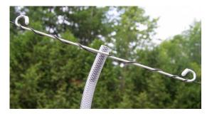
If the metal wire is straight, wrap the flying line in the same direction on either side of the flexible tubing so the spiral is continuous for the length of the wire. If the metal wire is bent around the tubing, this is not critical.
