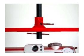
The lower end of the pendulum shaft has two holes for cotter pins. Both are important to secure the rig.
