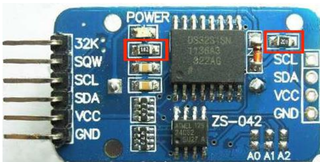
Remove these two resistors from the real-time clock board. (These photos are from Ed Mallon.)
