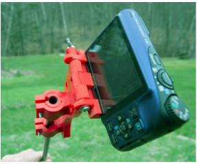
The back of the camera is snug against the lip to prevent rotation. The bushings are in place to accommodate the penultimate pole section.
