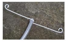
Bend the ends of the wire into almost closed loops. Use pliers with the noses taped to protect the vinyl.
