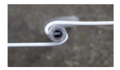
Bend the wire as shown (pliers are not needed). This is important to prevent the wire from rotating.
