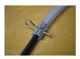
The larger cotter pin can lock the shaft in one of three positions.
